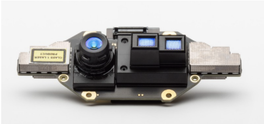
Figure 7.6: Depth Sensor: The Azure Kinect DK depth camera. Image taken from Microsoft [6].
