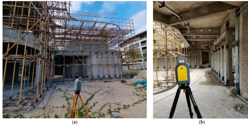
Figure 7.3: Laser scanning. A laser scanner is used to scan point clouds from a construction field. Image taken from [4].
